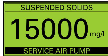
Figure 23 Service Air Pump Fault Message
