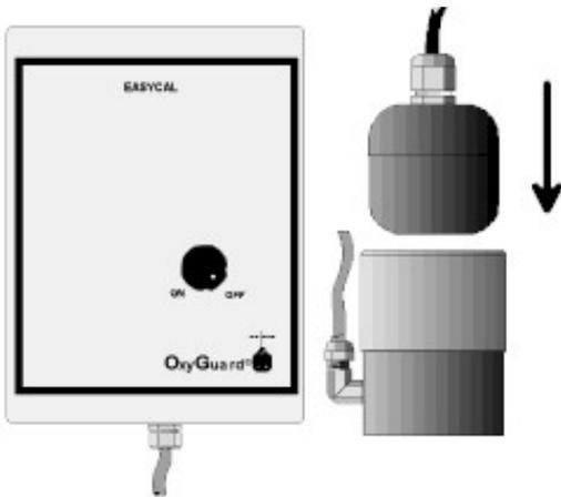
To use the EasyCal, lift the probe from the water, wipe the membrane, fit the EasyCal, return the assembly to the water, switch the EasyCal on and, as soon as the display is stable, press "CAL" and adjust the 840 Transmitter to the calibration value.
